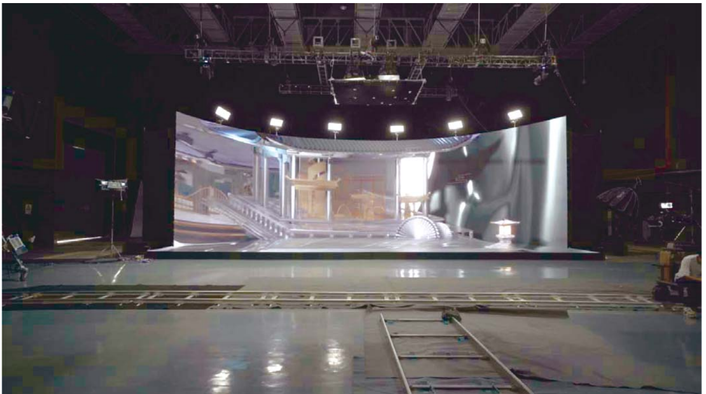
Figure 3 : Immersive LED screen for virtual shooting scenes
