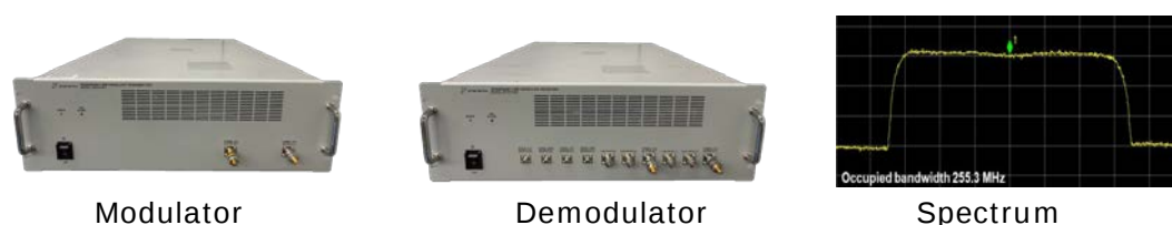
Figure 3-1: Wideband LDM-based modulator and demodulator
