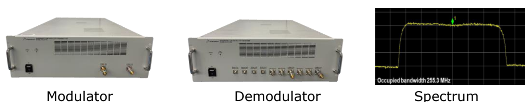
Figure 4-1 Wideband LDM-based modulator and demodulator
