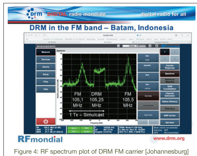
Figure 3: RF spectrum plot with DRM FM carrier inserted between two analogue FM carriers [Batam, Indonesia]
