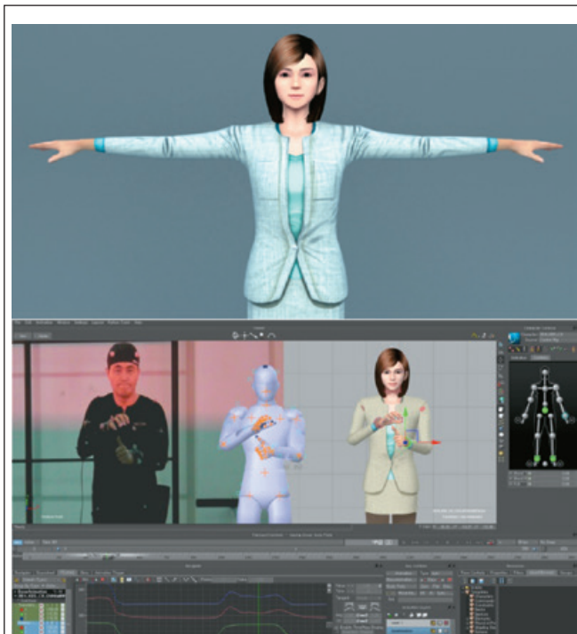
Figure 5: The avatar model and the captured motion applied to it
