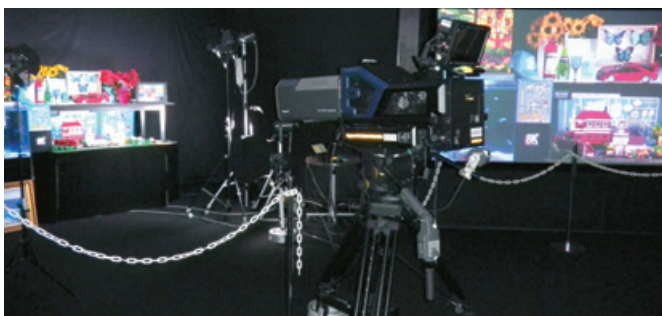
Figure 9: Demonstration of the UHDTV wide-gamut system colourimetry using an 8K video camera with the new prism and an 8K laser projector at NHK STRL Open House in 2013.
