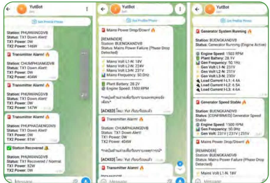
Fig. 3. Real-time automated Telegram notification logs pushed to engineers and technicians mobile endpoints.
