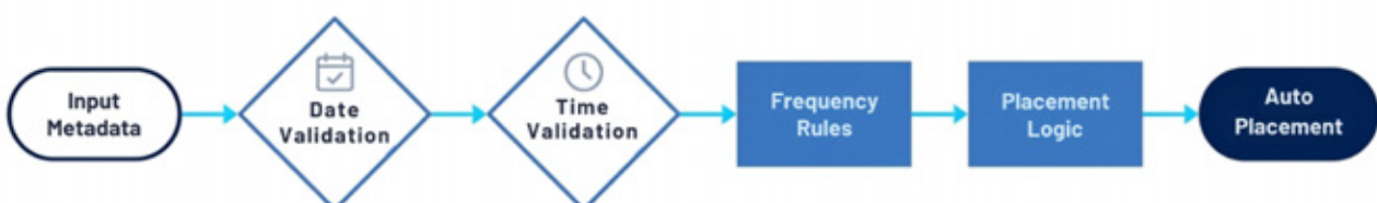
Figure 4. Rule-Based Scheduling and Autofill Logic.
