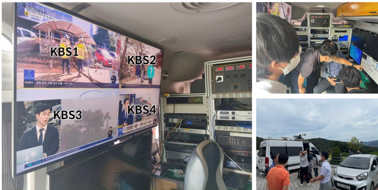
FIGURE 1.2.7 In the measurement vehicle, 4 UHD channels were successfully received at a rate of 15Mbps each, totaling 60 Mbps, using the prototype ATSC 3.0 MIMO transmitter and receiver.
